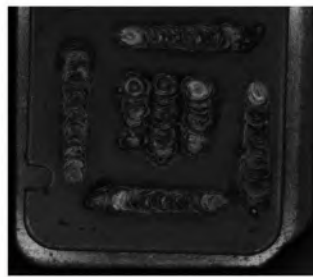
普通相机拍摄铝板焊接轨迹图 Aluminum plate welding path photo taken by the normal industrial camera.
